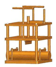
Impactor drop height to be set in accordance with calculation above, Specimen to be removed from pre conditioning and secured in test rig. Confirm specimen temperature with certified infrared thermometer then apply first impact within 60 seconds of removal from pre conditioning chamber and complete all impacts within 300 seconds. To achieve a WSX3 classification deformation will need to be less than 40% Record measurements of deformation results.
